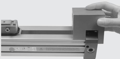
**1** Put the shock absorber support onto one end cap of the cylinder as shown in the picture.
