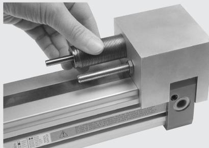
**7** Lock the shock absorber using the nut.
