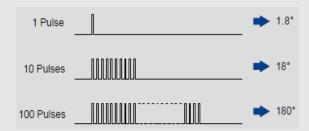
The pulse frequency (number of pulses per second measured in Hertz "Hz") determines the motor rotation speed.
