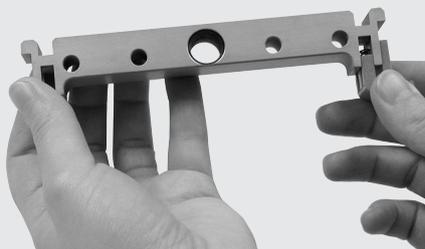
**6** Insert only one scraper (as prepared) into one of the two ends of the adapter.
