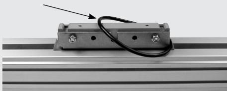
**1** Remove the O-ring seal from the carriage, taking care not to damage it.
