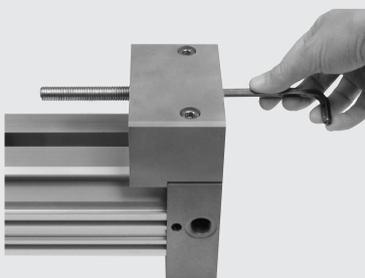
**3** Screw the stop grub screw in the desired position. Do not exceed the Bmax value shown in the table in fig. C.
