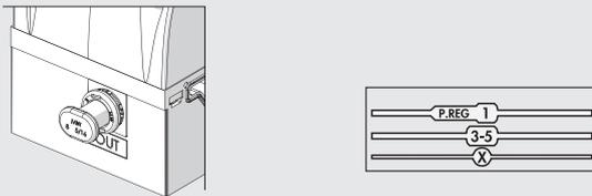
By applying a silencer on the exhaust port it is possible that the flow rates and response times may change. Periodically check the clogging of the silencer and replace it if necessary.
