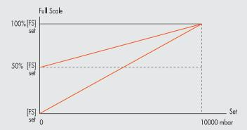
The minimum value which can be set with Keyboard Set is the Minimum Pressure value.
