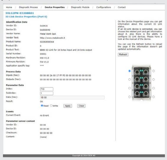
The Process Data area displays the state of Inputs and Outputs.
