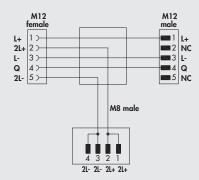
It can be used as supplementary power supply when the master module is not sufficiently powerful or to electrically separate the valve power supply when a machine safety guard is opened or an emergency stop button has been pressed.
