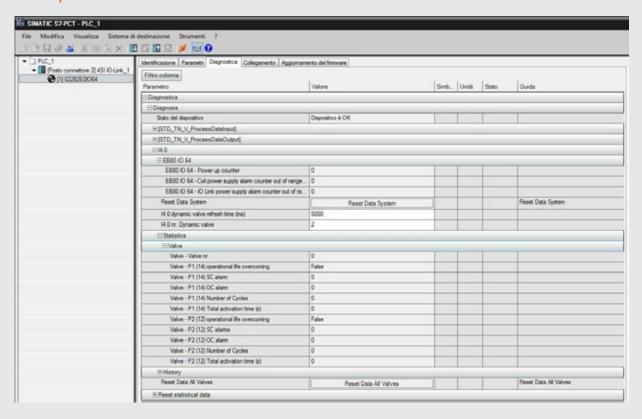
When replacing one or more valves, data can be reset using dedicated commands. The previous data are saved permanently in the related History fields and added to those saved with previous reset operations.
