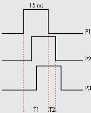
Total current consumption is equal to the power consumed by the solenoid pilots plus the current consumed by the electronics controlling the bases. To simplify the calculation, you can consider 3.2W consumed by each solenoid pilot simultaneously and 0.3W by each active solenoid pilot.
