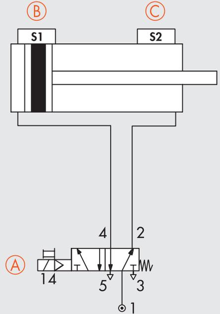
A = Valve in use, 5/2 one-pilot valve, pilot position on a base for two pilots = 7
