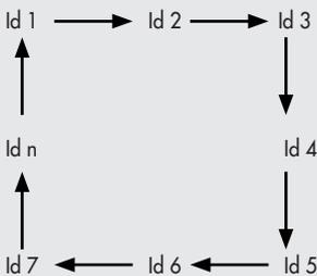
**Cycle counter:** showing the number of actuations of each solenoid pilot. When the number of cycles exceeds 60% average life, set at 30,000,000 cycles for the valves and 60,000,000 for pressure regulators, an alert comes on to **indicate that the average operating lifetime has been exceeded**.
